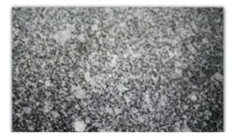
2) Insufficient Pretreatment: If too little pretreatment solution is applied the white ink will have a mottled appearance after printing(left). This is due to an insufficient amount of pre-treat required to keep the white ink layer on the surface (the ink soaks into the fibers of the shirt).
