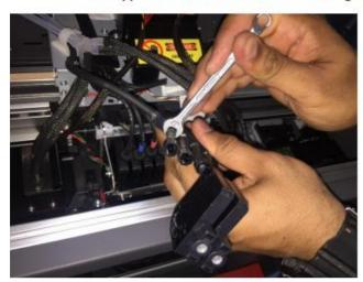
8- Block the holes by screwing a stainless steel M5X6mm screw with a silicon 'O' ring, so it seals properly and doesn't leak
