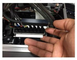
2- Undo the Damper holding bracket's thumb screws
