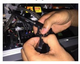
7- Undo the nipple from the white ink manifold using a 7mm spanner
