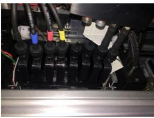
11- Trim the clear ink tube as per requirement and attached a 'Y' connector to it. If the clear is only going to be used in one channel then instead of connecting 'Y' connector, connect the tube direct to the damper
