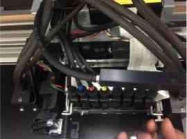
3- Remove the Damper holding bracket
