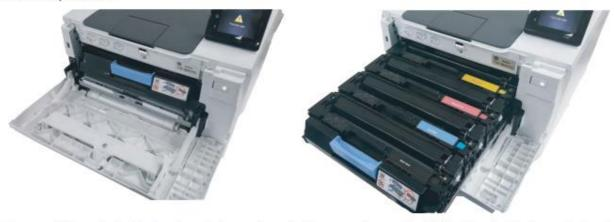
Lift the Toner cartridge out using the handle and place on its protective orange tray and inside the UV protection bag and place back in its box for storage:
