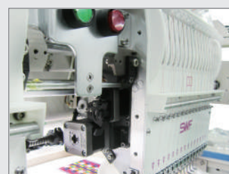
Adjustment of presser foot
